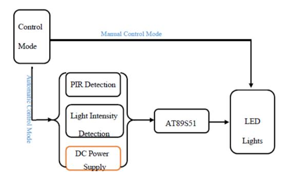
This system was designed to realize the goal of cutting down the amounts of electricity usage in people's daily life. The main enhancement deals with controlling lights that depend on current light intensity inside room and human existence for the purpose of gaining the optimal Efficiency of power saving.
