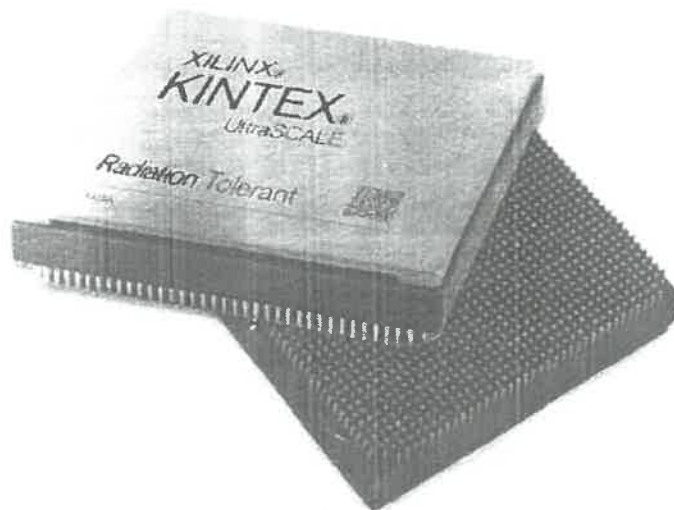
An FPGA IC belongs Xilinx Company
